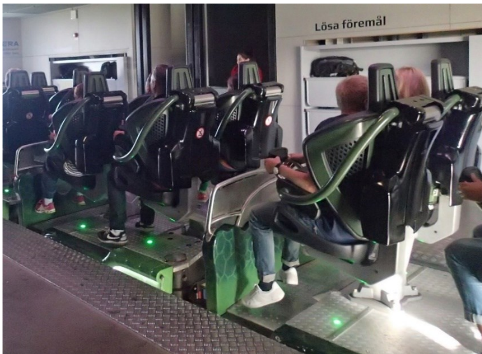
Figure 39: Open train design with floor level matching the station's floor (Helix – Liseberg)
