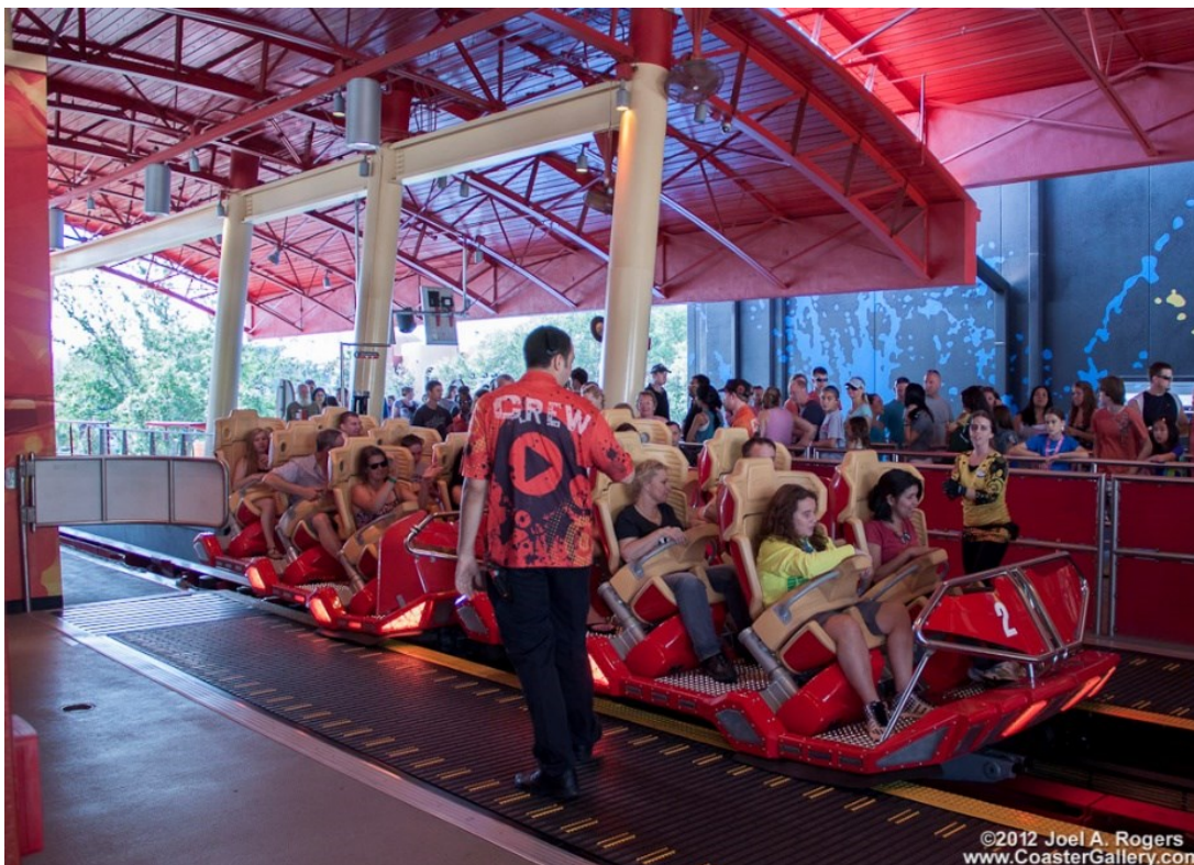
Figure 21: Moving station floor / conveyor belt [Fig. 15] (Hollywood Rip, Ride, Rockit – Universal Studios Florida)
