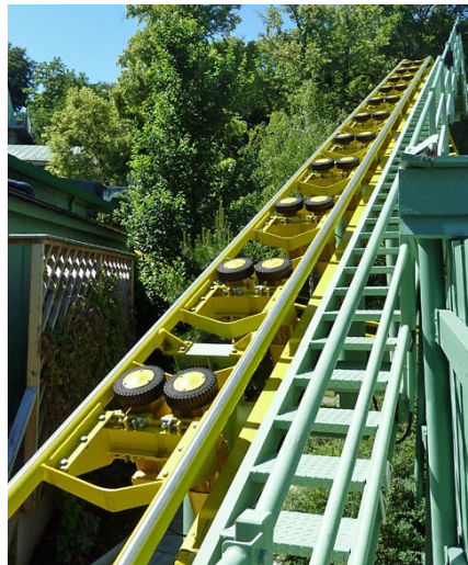
Figure 10: Tire drive lift hill [Fig. 8] (Rabalder – Liseberg)
