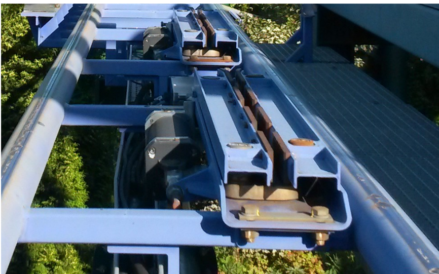
Figure 9: Double-jaw friction brake, operated by pneumatic pistons (Salama - Linnanmäki)
